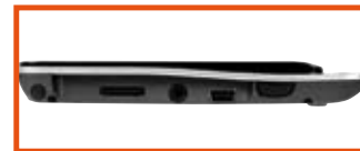
The left side of the unit has all the ports needed for its functions including a microUSB and mini USB port
